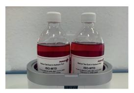
According to ISO 11171 the particles of a secondary calibration suspension must be counted by the use of a primarily calibrated master particle counter. Before this analysis, the suspension is homogenised via ultrasound.
