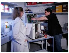
In order to assure constant measuring accuracy, automatic particle counters must be recalibrated at least once a year. PAMAS offers an After Sales Support for calibration and repair. This service may also be combined with a Service Contract. (Picture: PAMAS)
