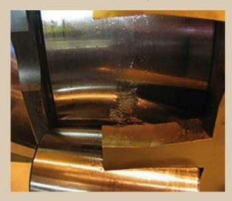
Unlike a contamination monitor, an automatic particle counter is able to provide information on abrasive particles. In a Finnish paper mill, the use of an automatic particle counter with 8 size channels revealed that mechanical components of the roller bearing were badly damaged. An exchange of the roller bearing limited further losses. (Picture: PAMAS)
