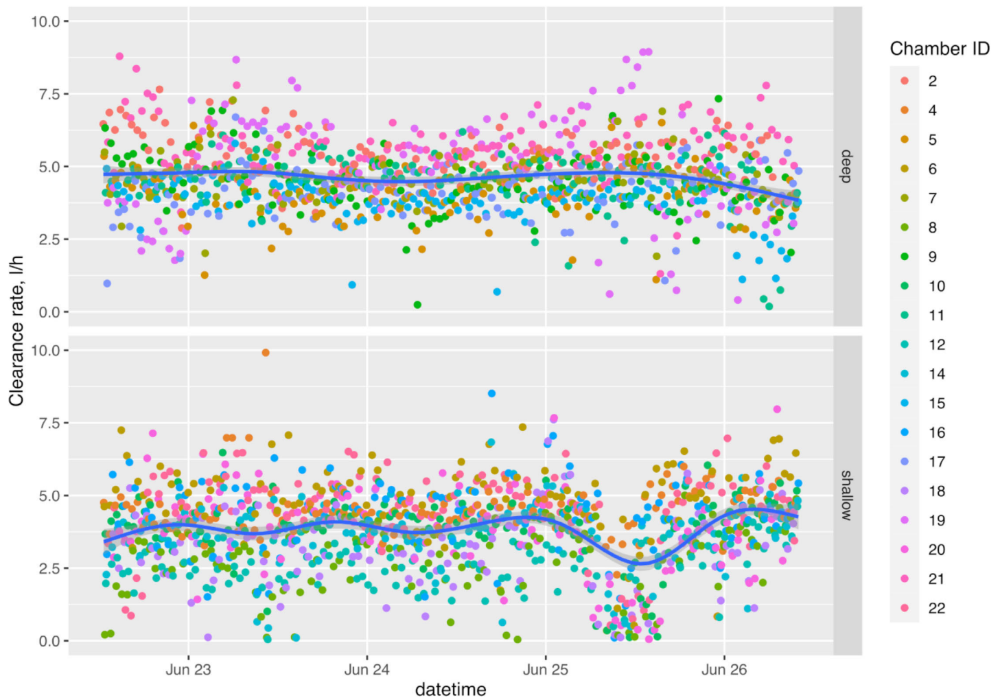
FIGURE 5. Individual clearance rates of Mytilus spp. of 4.5–5 cm shell length measured during the experiments. Deep and shallow treatments corresponded to the two depths at which water was pumped. Shallow pump was raised daily forcing environmental changes in the individuals receiving water from that pump.
