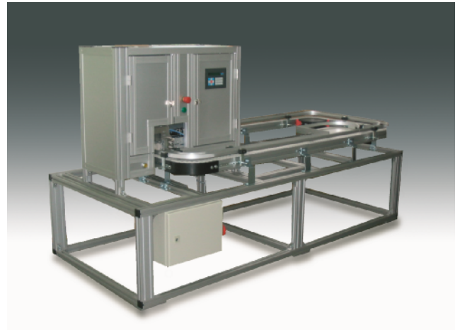
Picture 3: The second generation autosampling system PAMAS AS2, which was introduced in 2001, was equipped with a conveyor for concatenating systems. (Picture: PAMAS)
