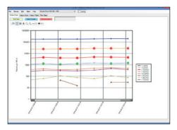
The software PAMAS POV shows particle measuring results in tables and graphs. The results are classified in size channels. On the graph, each size channel is displayed in another colour. The trend monitoring report can also be shown in a graph. (Screenshot: PAMAS)
