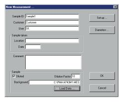
At the beginning of each new measurement, the operator can define the dilution factor in the software settings. The PAMAS PMA programme considers this factor during analysis and calculates the particle concentration of the originally undiluted sample. (screenshot: PAMAS)
