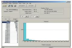
The software PAMAS PMA shows particle measuring results in tables and graphs. The results are classified in size channels. The number of displayed size channels can be defined by the operator in the software settings (screenshot: PAMAS).
