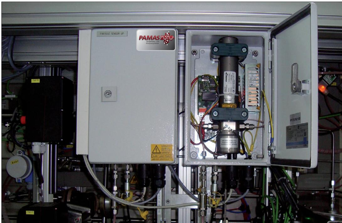
Due to its compact design, the online particle counting system PAMAS 4132 can be easily integrated into existing test rigs.
