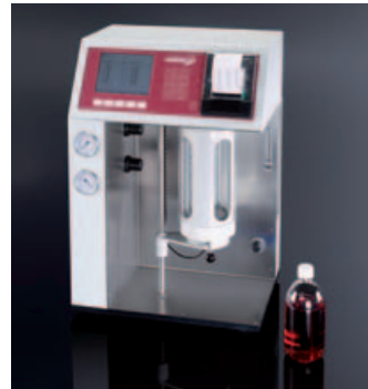
The measuring instrument PAMAS SBSS is a standard laboratory particle counter for high viscous bottle samples.
